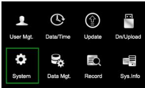
Press **M/OK** on the initial interface. Select **System** and press **M/OK**.
