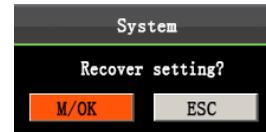
Press **M/OK** to reset; press **ESC** to exit.
