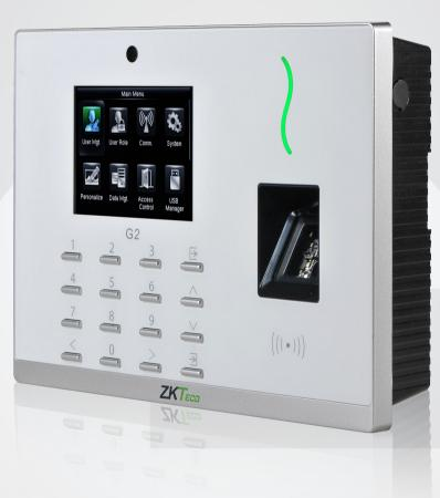
G2 fingerprint identification terminal features ZKTeco's innovative Silk ID fingerprint sensor. With 3D Neuron Fingerprint Verification Sensor-Activation and Anti-Interference technology, it precisely detects dry, wet, and rough fingerprints, and operates well under strong sunlight environment. With the latest core-board, the fingerprint capacity is enlarged to 20,000.
